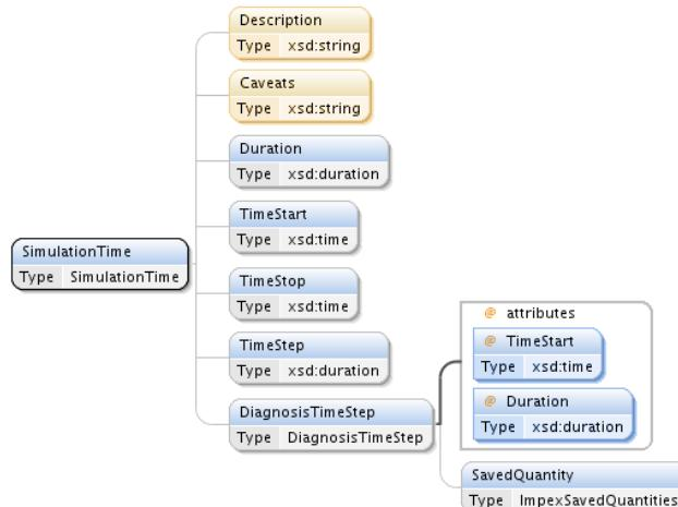
Figure 7 - SimulationTime element
