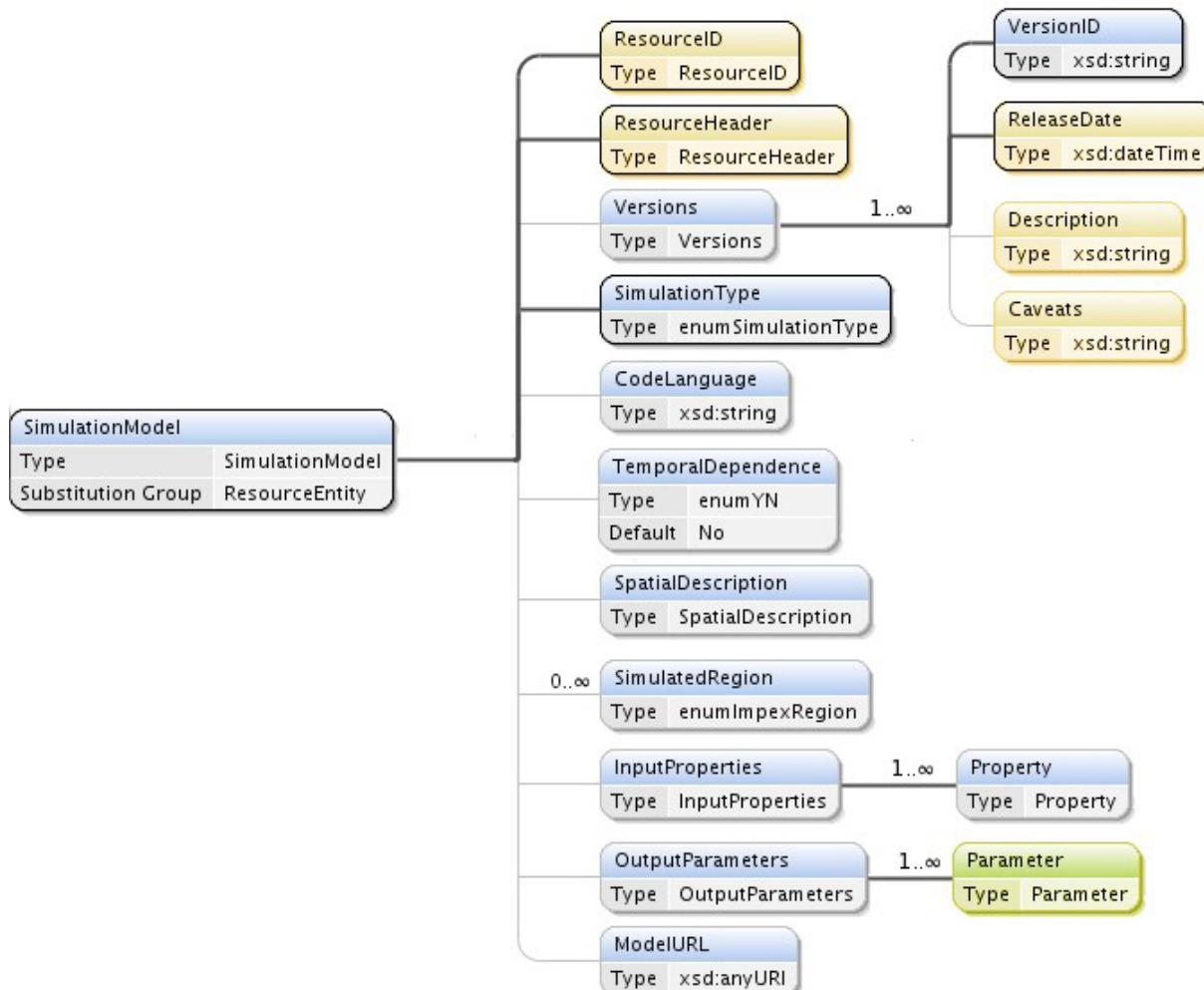
Figure 16 - *SimulationModel* element
