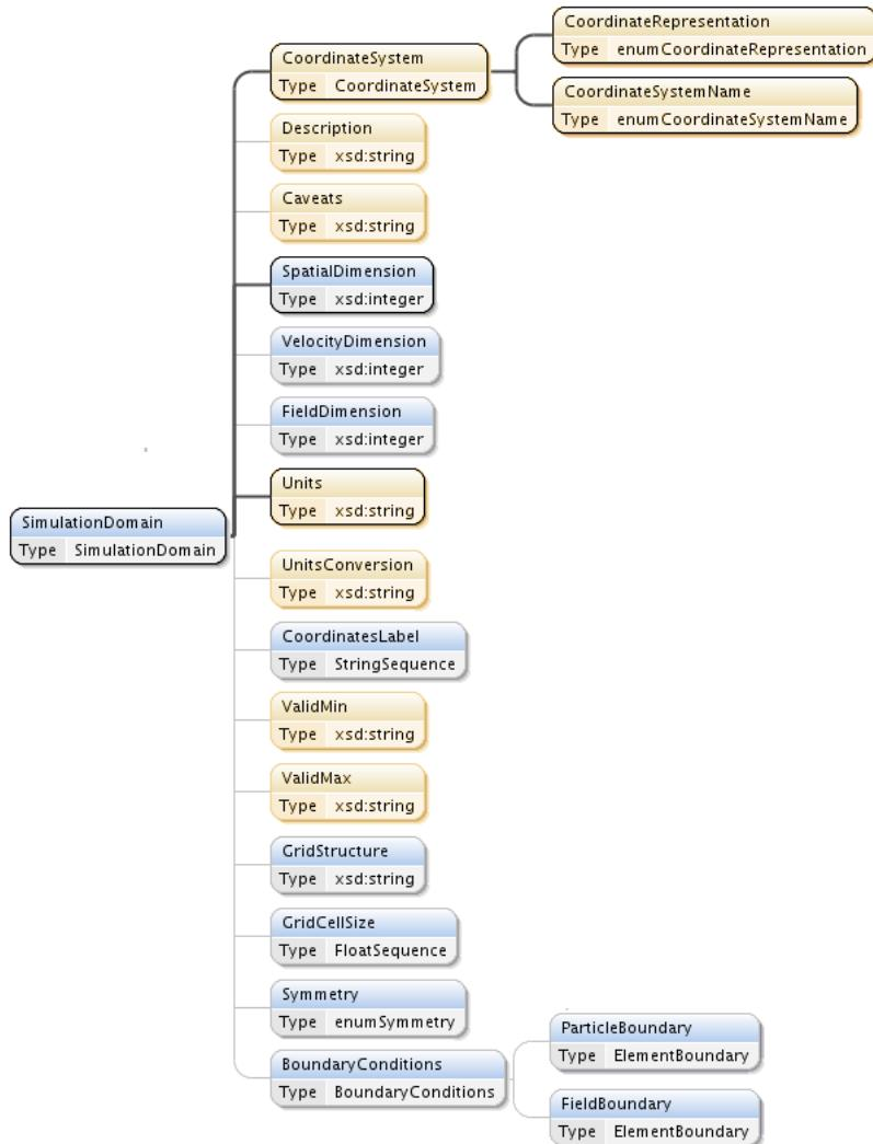
Figure 10 - SimulationDomain element
